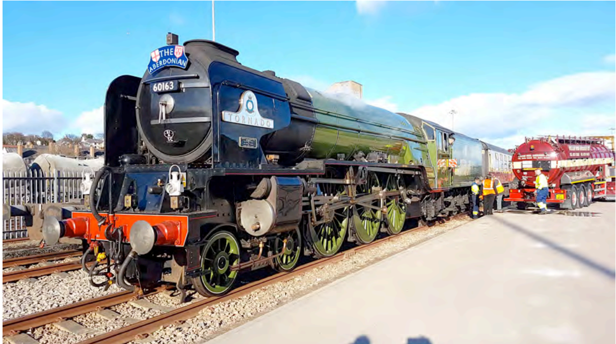
TORNADO BUNKERING WATER AT CRAIGINCHES KINDLY PROVIDED BY WILLIAN NICOL TANKERS SUPPLYING 27,000 LITRES FOR THE LOCO AND A SECOND TANKER FOR THE COACHES (PHOTOGRAPH – COURTESY OF CHRIS MAGUIRE)
